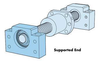
HepcoMotion BEK bearing housings are suitable for miniature ball screws. The housings are made from chemically blackened steel and contain a pair of matched angular contact bearings, to provide accurate radial and axial location for the ball screw. On installation, the locking nut should be fully tightened and locked in place using the grub screw. Standard machined 'Fixed Ends' fit into these housings (see Figure A on 9).
